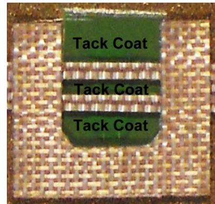
D) Curing the tack coat (partial curing)
